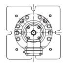
This special burner body has two sets of connections for mounting pilot or spark igniter and flame detector. This permits a variety of piping arrangements or redundant pilots and flame detectors. It is available only in -2 through-6-B burner sizes and is otherwise identical to a standard burner. For dimension information refer to Dimensions & Parts List 4422-5.
